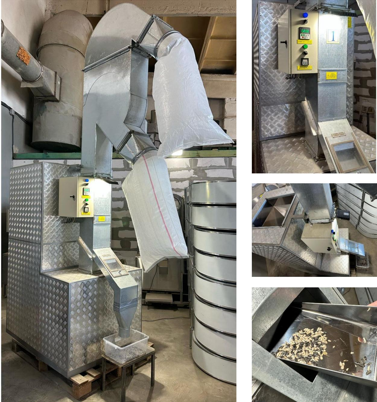
**Fig. 1.** The general appearance of the experimental prototype of the column-type aerodynamic separator
