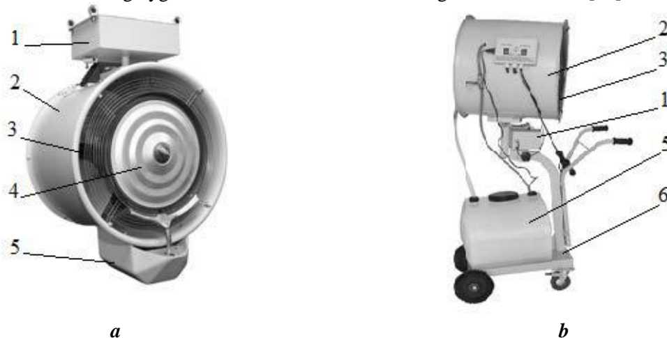
Fig. 3. Centrifugal air cooler: a – stationary; b – mobile; 1 – drive mechanism; 2 – housing; 3 – fan; 4 – disk; 5 – tank; 6 – trolley
