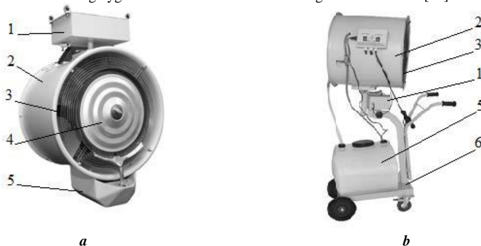
Fig. 3. Centrifugal air cooler: a – stationary; b – mobile; 1 – drive mechanism; 2 – housing; 3 – fan; 4 – disk; 5 – tank; 6 – trolley
