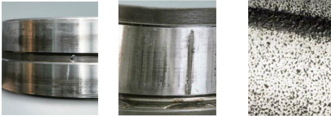
Fig. 2. Appearance of fretting-corrosion processes in rolling mills [7]
