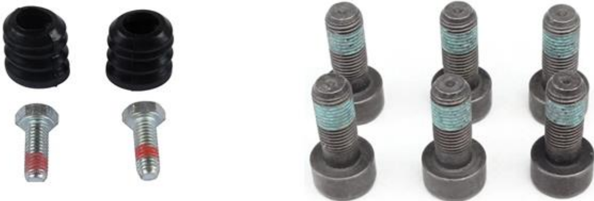
Fig. 1. Examples of the use of polymeric materials on threaded surfaces
