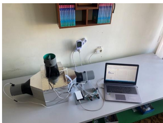
Fig. 2. Schematic diagram (a) and general view (b) of the laboratory test bench for investigating an indirect evaporative heat exchanger
