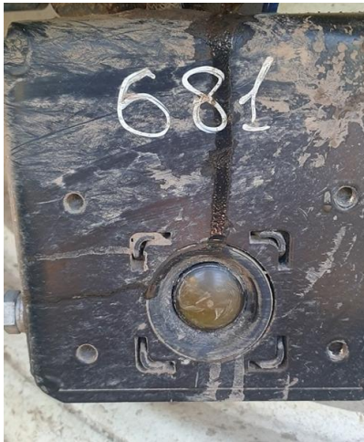
Fig. 3. Test 1 – radar condition without using air blowing
