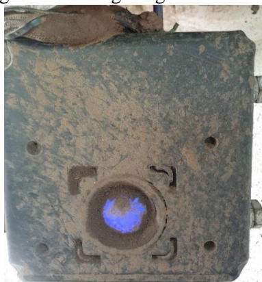
Fig. 9. Test 4 – radar condition without using air blowing
