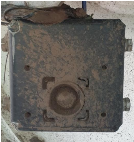
Fig. 5. Test 2 – radar condition without air blowing
