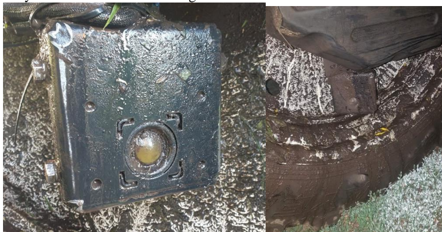
Fig. 7. Test 3 – radar condition without using air blowing
