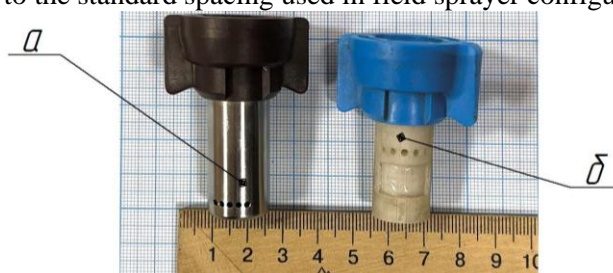
Fig. 2. Jet nozzles: a – RD.05.SD5-b; b – combined type
