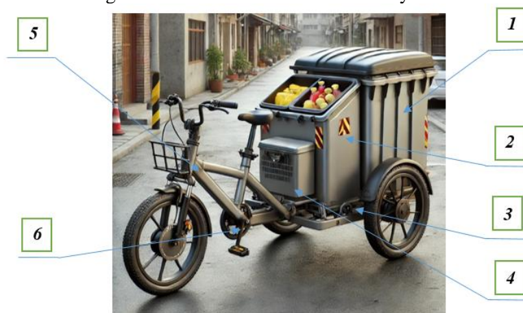
Fig. 7. A current example of technologies and trends for the future use of track bikes, which would be designed for transporting solid household waste: 1 – tank for SHW (solid household waste); 2 – additional compartment for other types of materials; 3 – platform of the bikes – trucks, on which the SHW tank is placed; 4 – battery; 5 – bikes – trucks; 6 – mechanism for driving the pedals of the bikes – trucks wheels.
