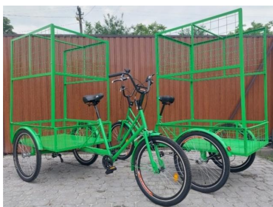
Fig. 3. Rymar Marsel New cargo bike of the "Flower" brand, which can be used by housing and communal services workers, gardeners, hotel and country business owners for transporting heavy, oversized cargo – with a load capacity of up to 200 kg [2].
