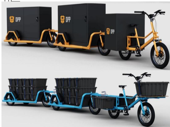
Fig. 4. French electric cargo bike-train “Pelican eTrain”. A modular monster that can be equipped with two electric trailers to transport up to 500 kilograms of cargo, the total volume is 3000 liters [14]
