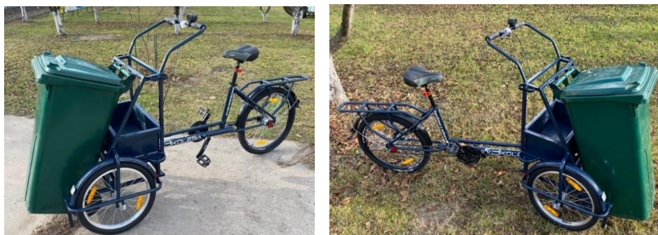
Fig. 2. Cargo tricycle with the possibility of installing a garbage can in front for organizing cleaning, tidying and servicing of objects of the Cargo brand "Trash-Bike" [1]
