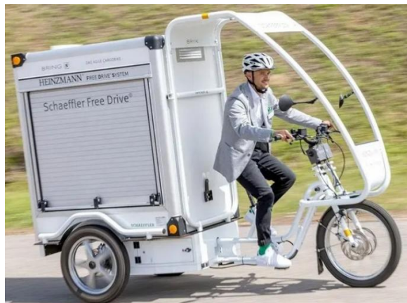
Fig. 5. Electric cargo bicycles with a chainless Free Drive drive system that can be used to deliver food, mail, and medicine in the city center [15]
