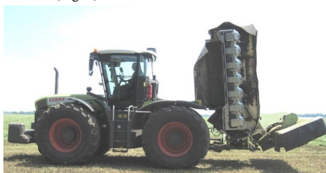
Fig. 1. Power tool "XERION 3300" with a combination of mowers DISCO 8600DUO in work (a) and when moving (b) Source: author's proposal
