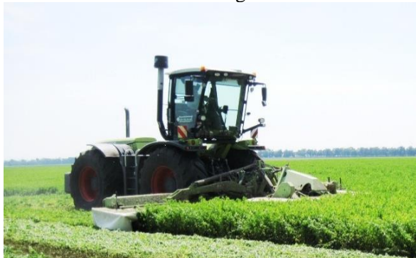
Fig. 1. Power tool "XERION 3300" with a combination of mowers DISCO 8600DUO in work (a) and when moving (b) Source: author's proposal
