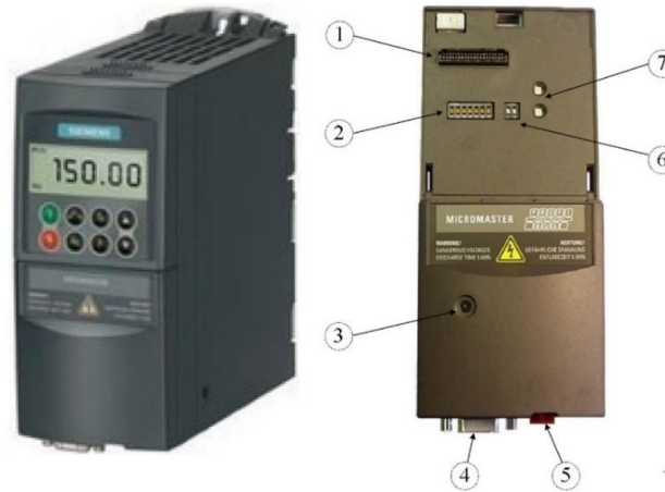
Fig. 2. External view of the Siemens Micromaster 440 frequency converter and PROFIBUS communication module: 1 – control unit connector, 2 – PROFIBUS address switches, 3 – communication module status LEDs, 4 – communication module interface, 5 – external 24 V power supply connector, 6 – service switches, 7 – MICROMASTER4 status LEDs
