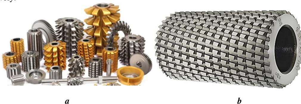
Fig. 11. Types of cutters for gear cutting machines: a) – corn; b) – a shaper layer.
