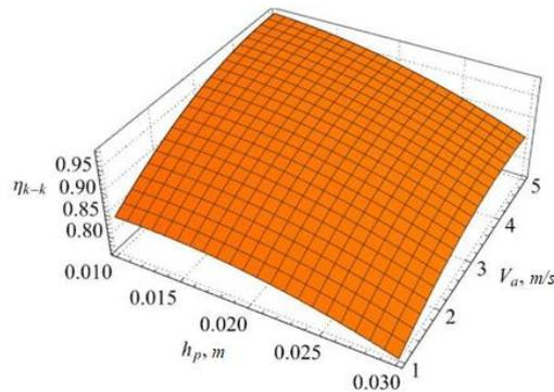
Fig. 5, Dependence of the content of sunflower kernels in the area of the kernel collector  $\eta_{k-k}$  from the height of the waste layer of the supplied sunflower seed mixture,  $h_p$  and air flow speeds  $V_a$
