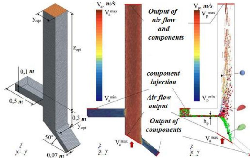
**Fig. 2. Modeling scheme of waste separation of sunflower seed mixture in a pneumatic separation channel**
