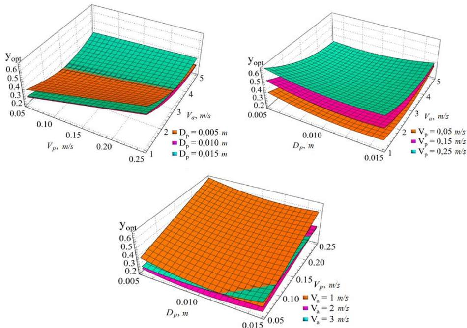
Fig. 3 Dependence of the horizontal flight distance of the components (sunflower husks and small particles)  $y_{opt}$  from the effective diameter  $D_p$ , component feed rates  $V_p$  and air flow speeds  $V_a$
