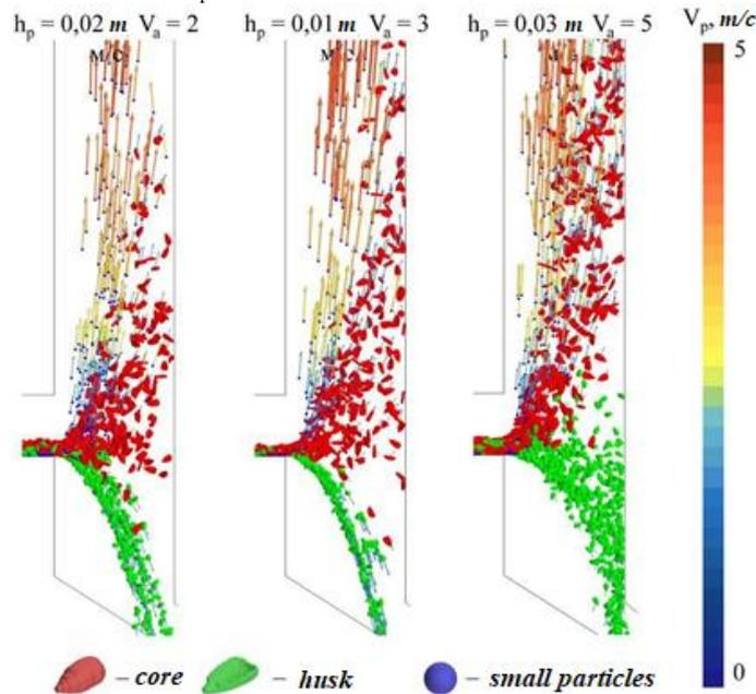
Fig. 4. Distribution of seed mixture waste components in the pneumatic separation channel
