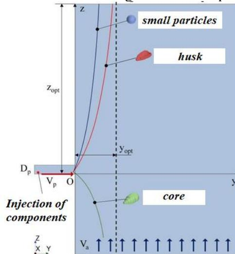
**Fig. 1. Scheme of modeling the movement of waste components of the sunflower seed mixture in the pneumatic separation channel**
