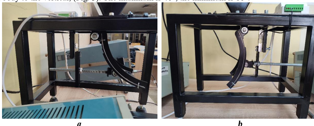
Fig. 3. View of the angle of inclination of the working body to the vertical: a – 40^\circ ; b – 10^\circ
