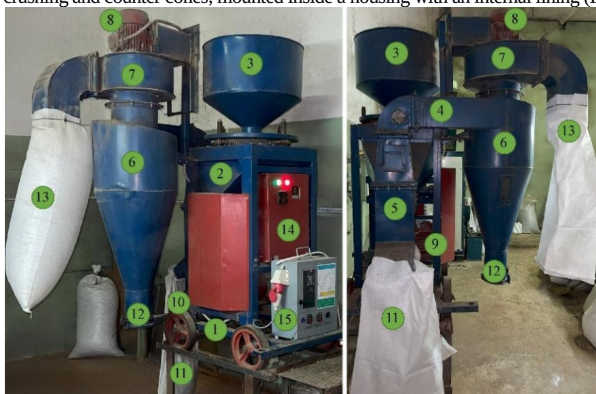
Fig. 1. Test bench for studying the castor seed cleaning machine:
