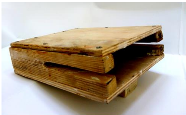
Fig. 3. Device for removing plaster casts of cultivator blade blades.
