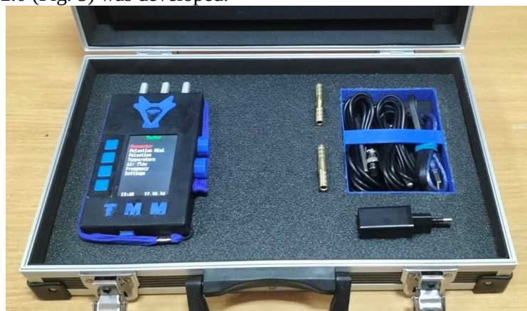
Fig. 5. General View of the Milking Unit Tester v.2.0
