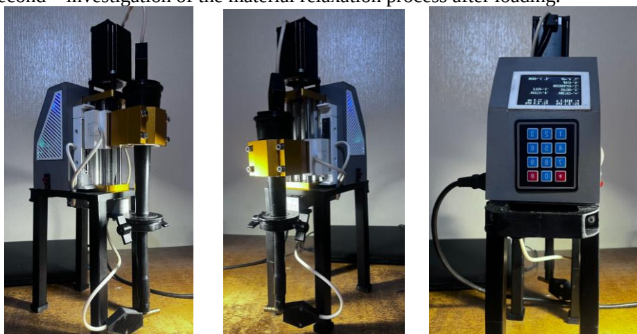
Fig. 7. General View of the Teat Rubber Testing Stand
