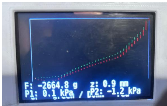
Fig. 8 Graph of changes in the condition of the teat rubber, green – tension, red – compression
