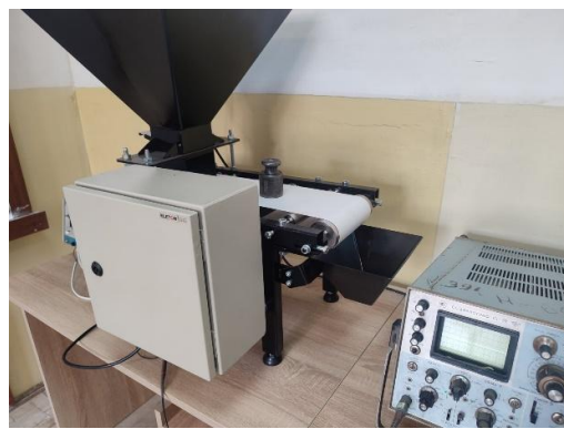
b – calibration with a reference load
