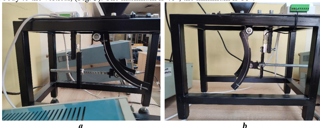
Fig. 3. View of the angle of inclination of the working body to the vertical: a – 40°; b – 10°
