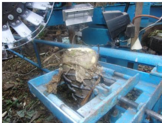
Fig. 3. Fixing the root crop in the frame of the “moving field”: a – device diagram; b – general view of the “moving field” frame with the root crop fixed
