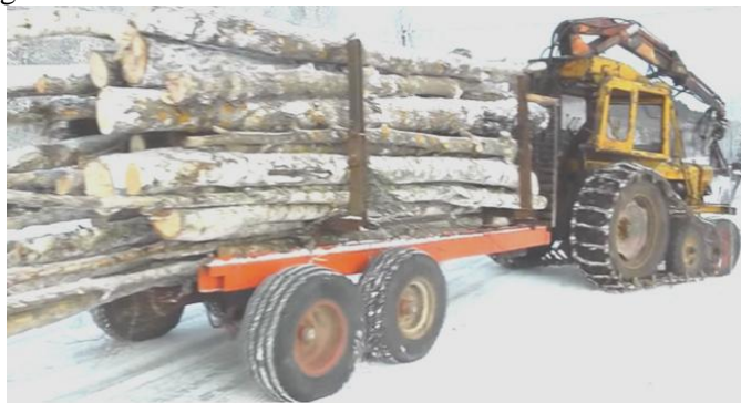
Fig. 2. Forwarder based on a tractor with a half-track
