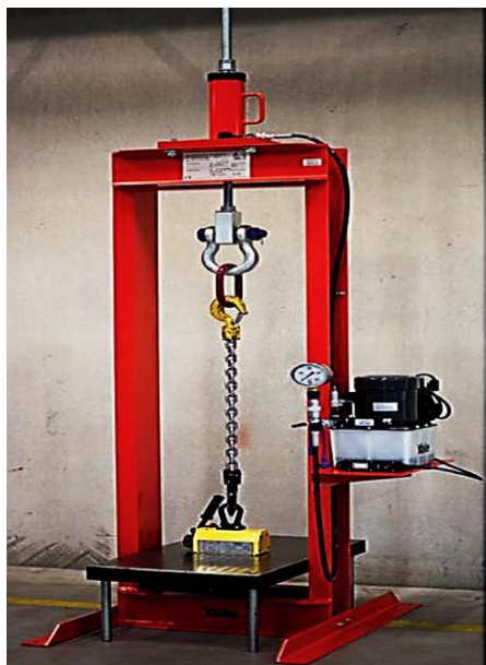
Fig. 1. Stand for testing round-link load chains
