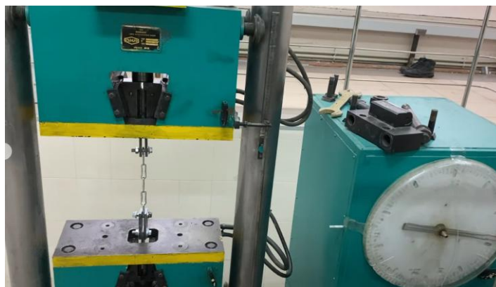
Fig. 4. R-50M1 tensile testing machine
