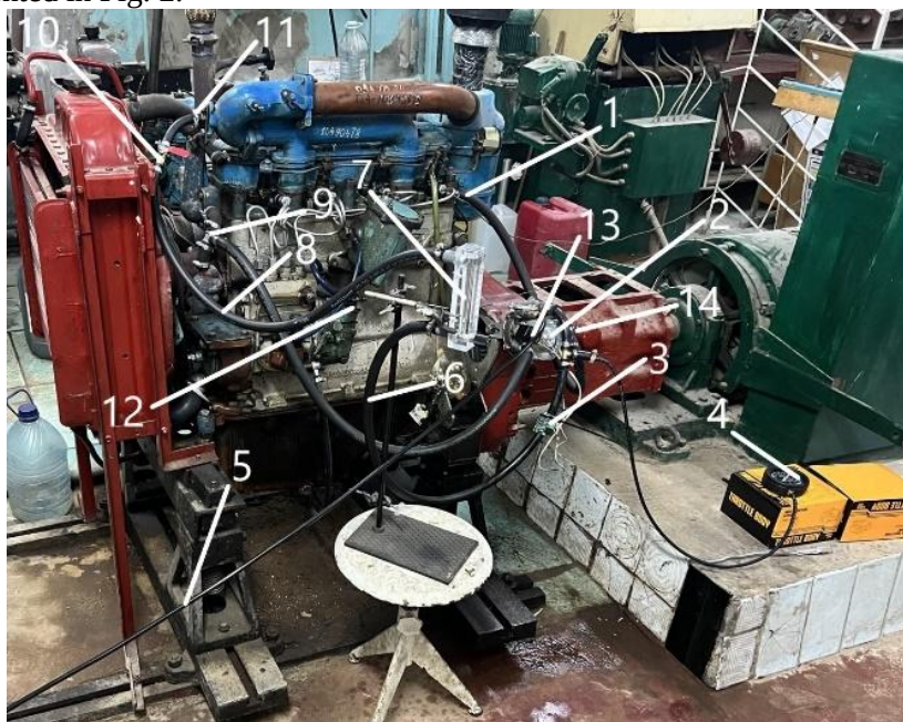
Fig. 2 Experimental installation with gas cylinder equipment:
