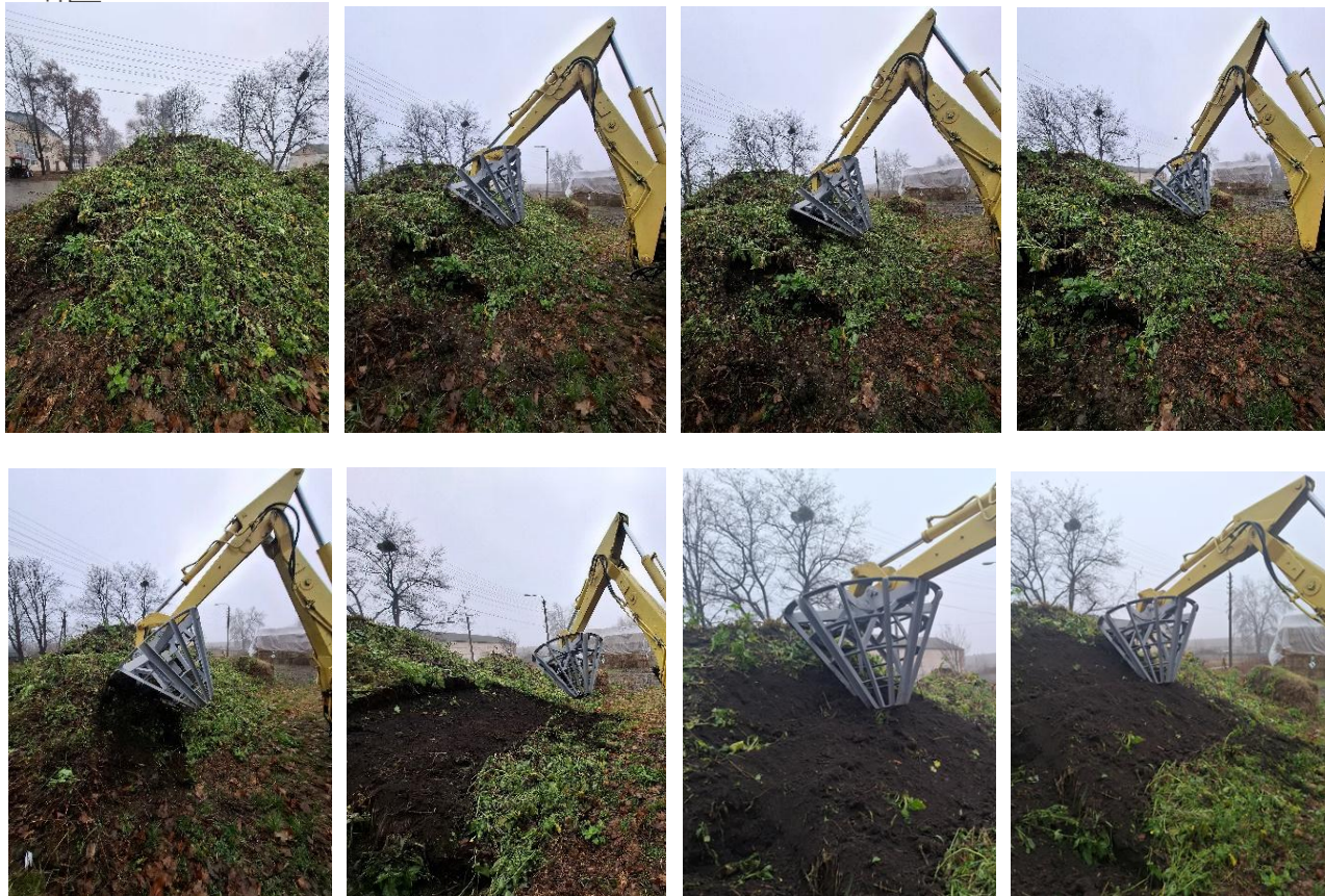
Fig. 4. Storyboard of the process of cleaning the damaged soil layer with a working body
