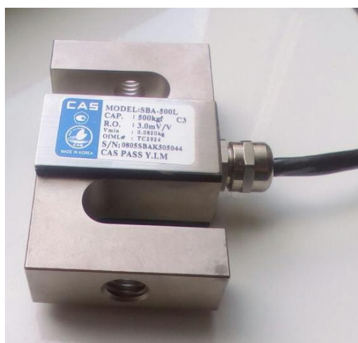
Fig. 3. General views of the tensile-compressive strain gauge CAS SBA-a00L (a) and the electronic dynamometer DE-2.0-0.5 (b), which were used to measure the soil shear force
