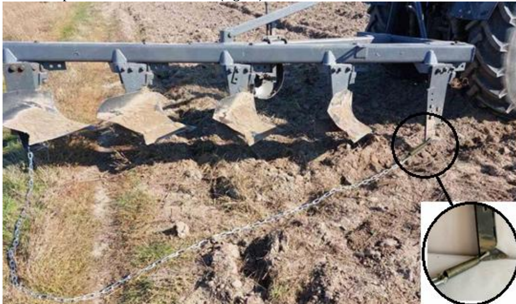
Fig. 11. Combined tillage unit consisting of: PLN-5-35 plow (modernized) and flexible chain soil deepener
